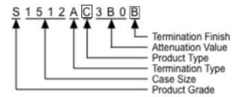
Fixed chip attenuators with termination finish code B (tin-lead solder over nickel barrier) contain the SVHC material lead. Attenuators with termination finish code B **DO NOT** comply with REACH.
