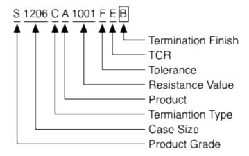
Precision thin film chip resistors with termination finish code B (tin-lead solder over nickel barrier) contain the SVHC material lead. Resistors with termination finish code B **DO NOT** comply with REACH.
