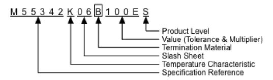
MIL-PRF-55342 chip resistors with termination material U (Platinum/Gold) contain the SVHC material cadmium as cadmium oxide and lead oxide.
