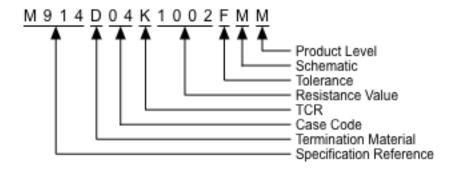
All MIL-PRF-914 surface mount resistor network products contain lead in the tin-lead solder termination finish and contain lead oxide in the resistor and glass materials. These products **DO NOT** comply with REACH.
